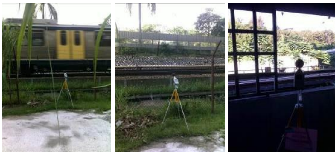
Plate 7-1 LRT pass-by noise measurements at Jalan Hang Jebat and Raja Laut
