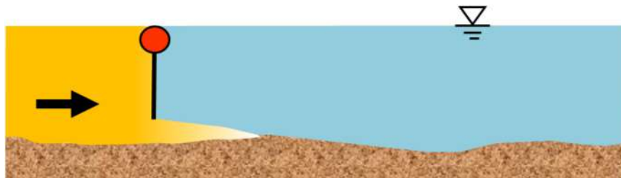
b) With silt curtain
