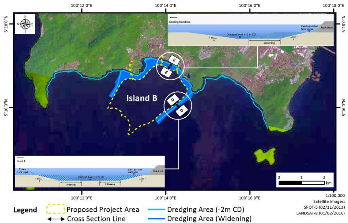
F5.42 Proposed channel widening works in Phase 1
