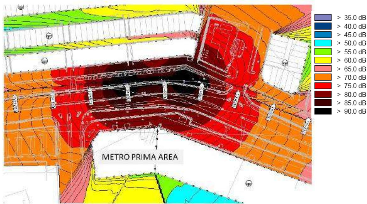
Chart 7-5 Noise Propagation from Piers Bored Piling (with 4m hoarding) at Vista Mutiara area
