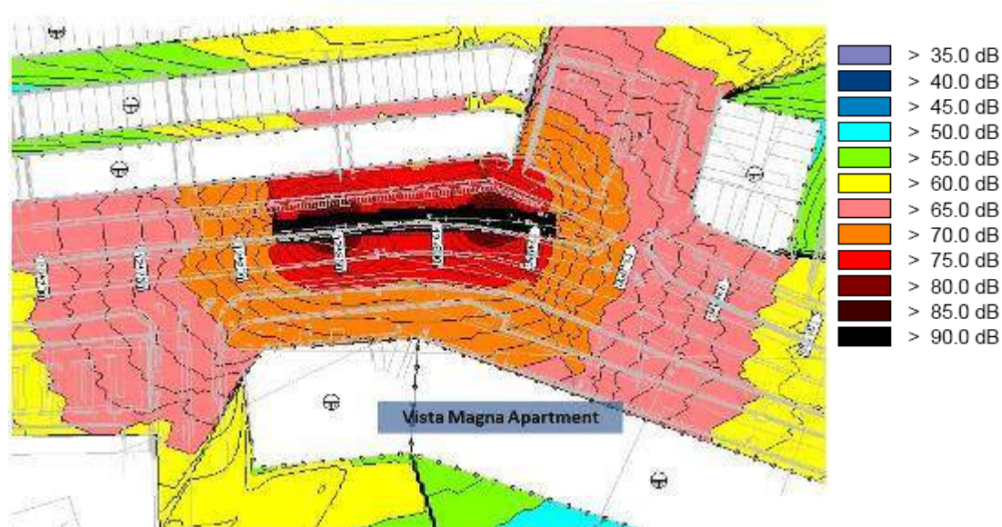
Chart 7-34 Noise Contours From Piling (2 Piling Machine) With 12m Noise Barrier
