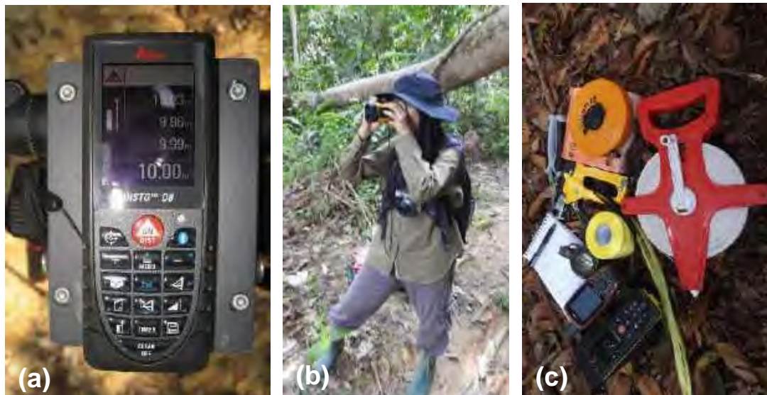
Figure 6.37 : a) Leica Disto D8 Laser Rangefinder was used to measure horizontal terrain distance b) Nikon Forestry was used to measure tree height c) Equipment for plot establishment and inventory
