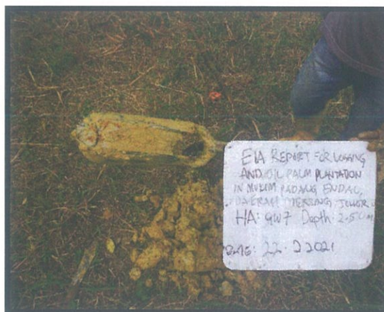
Photo 20: Augered Sample at depth 2.50m for GW7
