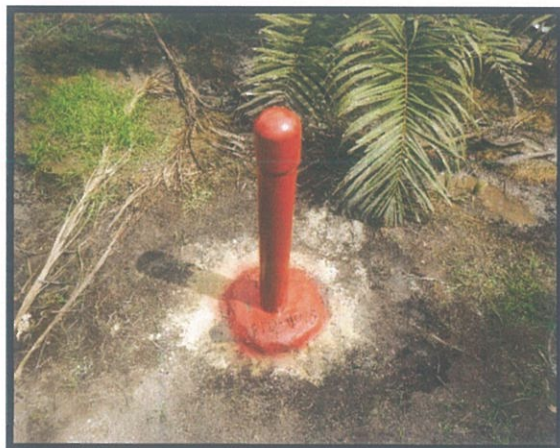
Photo 8: Completed Standpipe Piezometer at GW2
