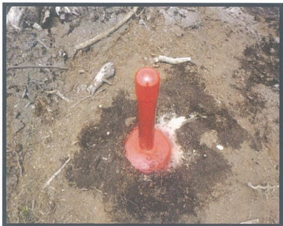
Photo 17: Completed Standpipe Piezometer at GW6
