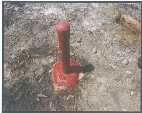
Photo 14: Completed Standpipe Piezometer of GW5
