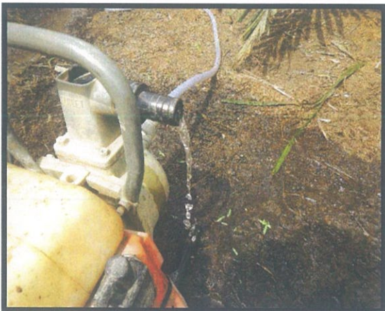
Photo 7: Water sample collection after purging
