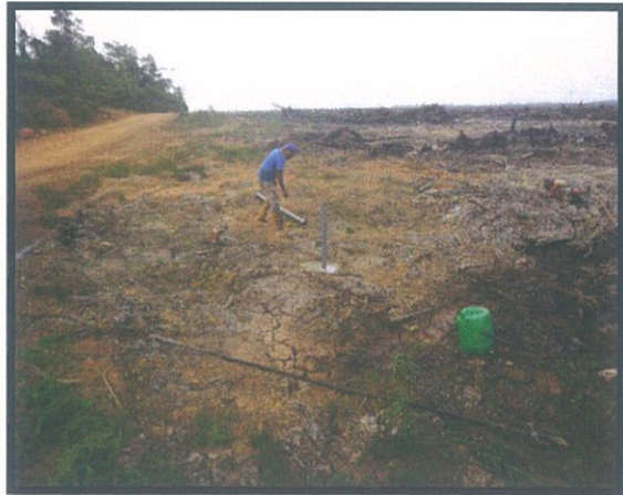
Photo 10: Installation of Standpipe Piezometer
