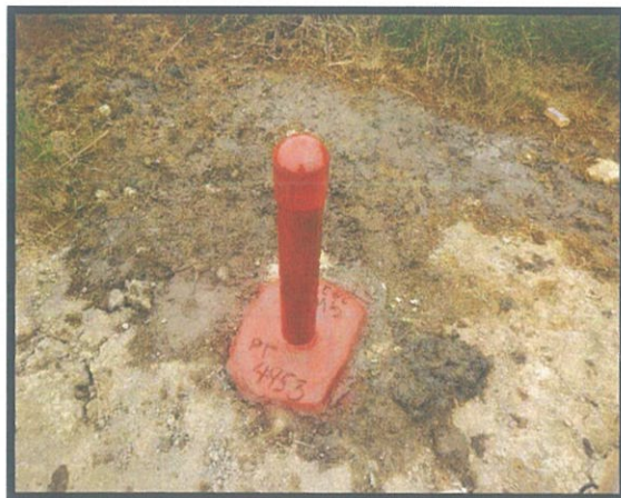
Photo 12: Completed Standpipe Piezometer for GW4
