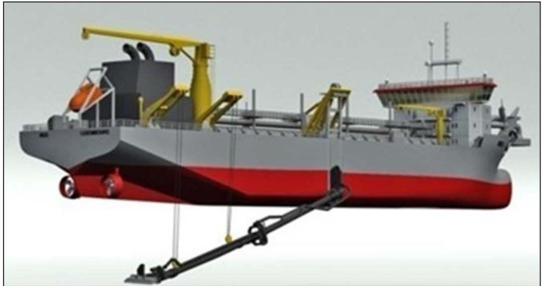
Figure 5.12 An example of a trailing suction hopper dredger (Source: PIANC /10/).
