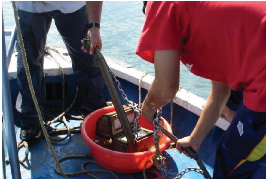
Photo 3.20 Van Veen Grab Sampler used to retrieve top sediment samples.
