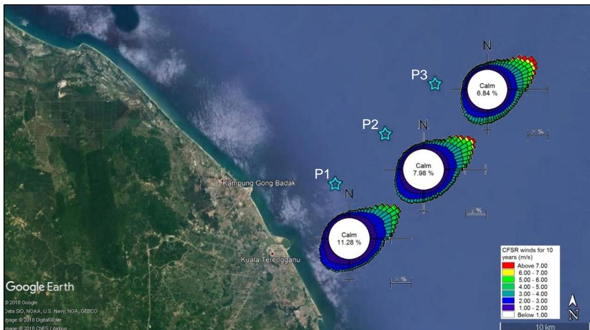
**Figure 12: Monthly wind roses at three (3) extraction points (source: DHI)**
