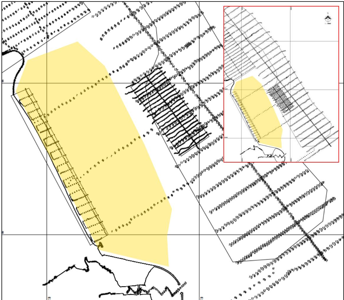
**Figure 4: Bathymetric survey of the project site before reclamation works (source: DHI)**
