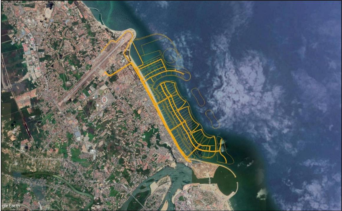
**Figure 2: Layout of the proposed reclamation area (source: DHI)**
