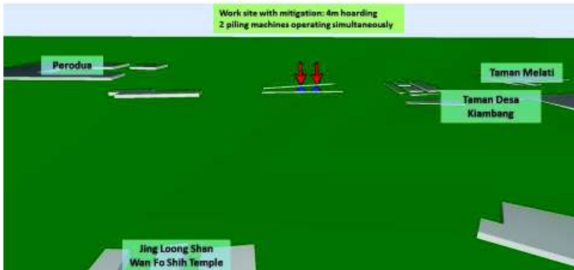
Chart 7-18 : Noise Model of Work Site at Serendah Station with 4m hoarding
