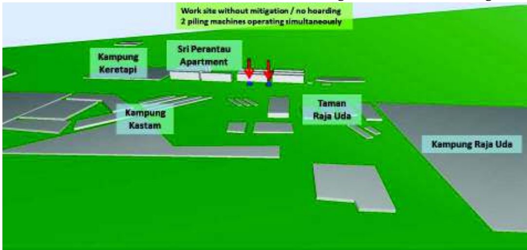
Chart 7-23 : Noise Propagation from Piling at Port Klang Station without Mitigation
