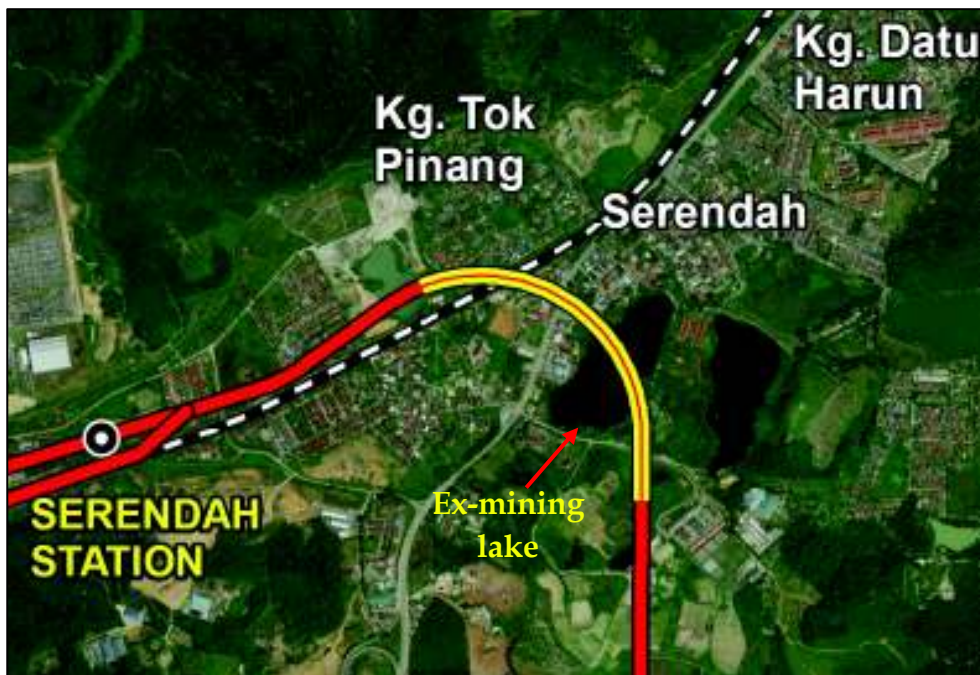
Chart 7-38a : Alignment crossing limestone and mined out areas
