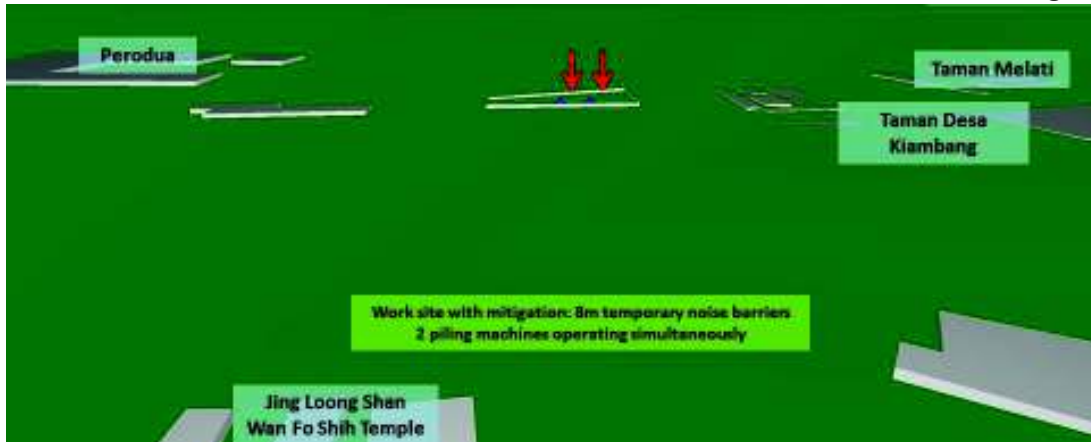
Chart 7-20 : Noise Model of Work Site at Serendah Station with 8m hoarding
