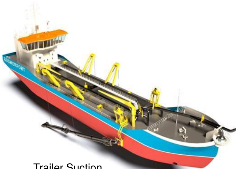
Trailer Suction Hopper Dredgers
