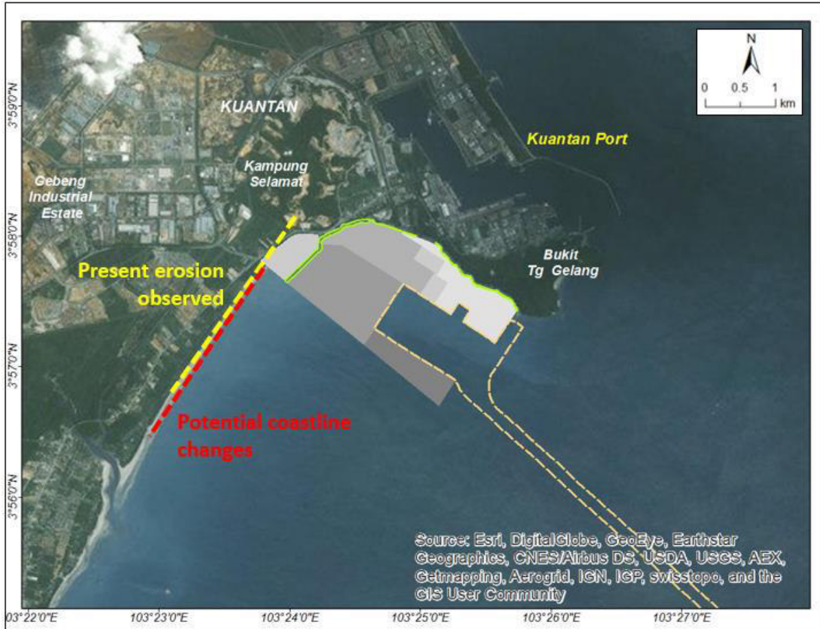
Figure 7.2.95: Predicted potential coastline changes after the completion of project
