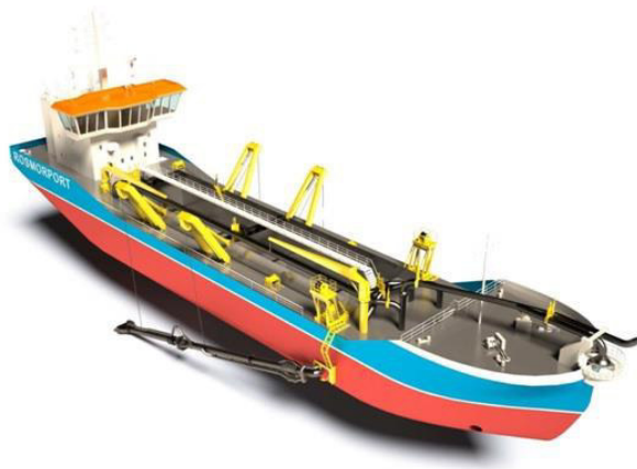
Plate 5.3.5: Typical view of a TSHD with dredger head
