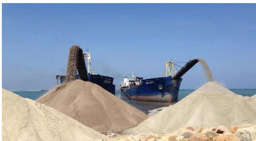
Plate 5.3.1: Conveyor belt system from sand carrier
