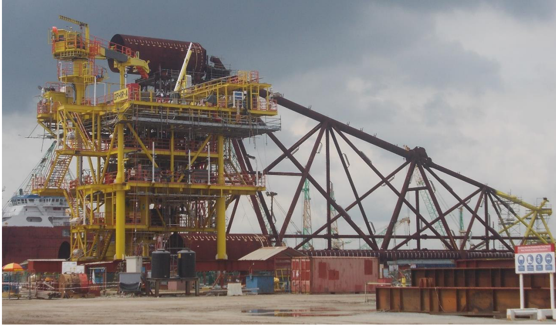
Plate 5.3.10: An example of product (offshore topside module) being fabricated and build at fabrication yard.
