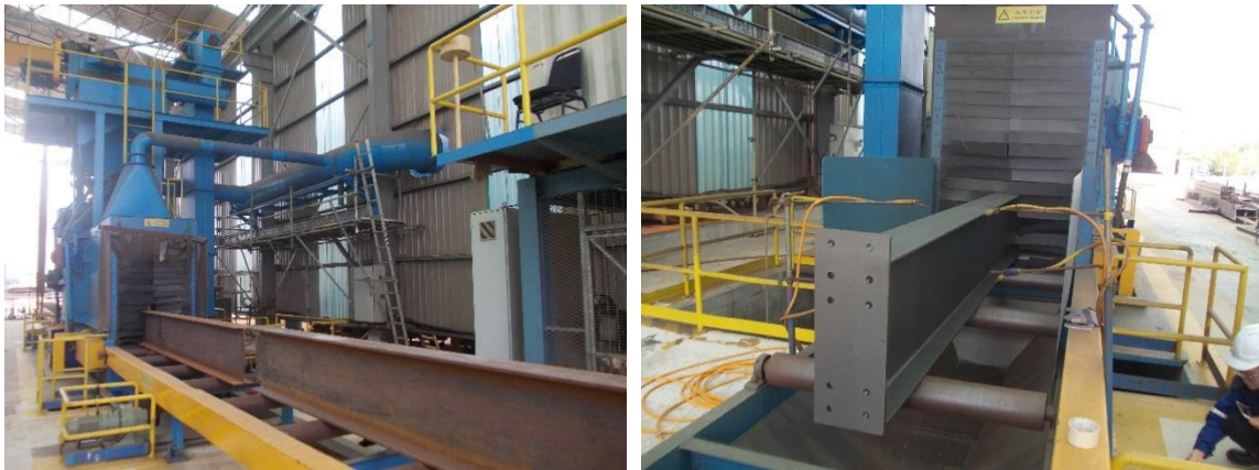
Plate 5.3.7: Before and after sand blasting products.
