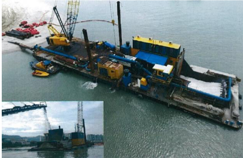
Plate 5.3.2: Sand transfer pump barge
