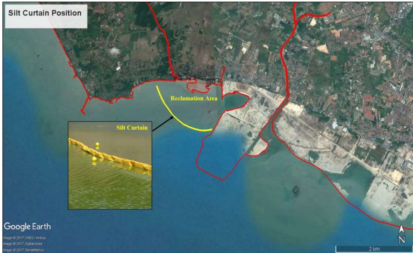
Figure 23: Silt Curtain Position during Reclamation Work
